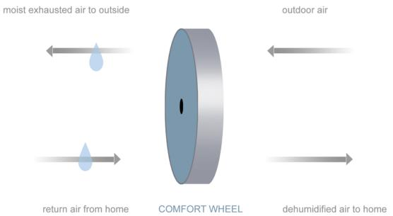
The revolutionary new technology of NovelAire's Comfort Wheel is specifically designed to maximize moisture removal and comfort in your home. The Comfort Wheel rotates slowly while simultaneously absorbing the moisture from your home. The moisture-laden wheel then rotates into the outdoor air stream where the unwanted, excess moisture is discharged outdoors. This energy efficient process provides greater comfort and lower cooling bills.
