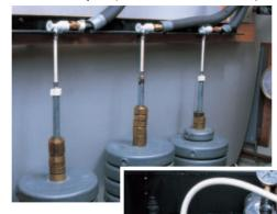
Intermittent shock testing (125psi - 180psi, 140°F, 30,000+ cycles).
