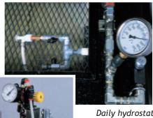
Daily hydrostatic testing (shows 1400psi-actual pressure).
